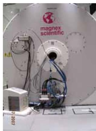
Figure 6: 700 MHz (16.4 T) magnet with 260mm bore
